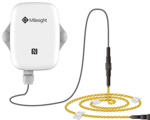
EM300-ZLD is a compact zone leakage detection sensor for detecting large area presence of water (or other liquids) and transmitting alarm using LoRaWAN® technology. With this low power consumption technology, EM300-ZLD can work up to 5 years with 4000 mAh battery. Combining with Milesight LoRaWAN® gateway and Milesight IoT Cloud solution, users can manage all sensor data remotely and visually and receive alarms via mobile APP.
