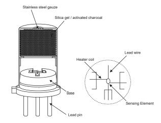
Figure 1 - Sensor structure
