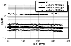
Figure 8a - Long term stability for methane sensing (Ro = Rs in 3000ppm of CH4 at Day=0, VH =0.9)
