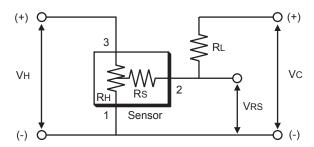
Figure 4 - Basic measuring circuit
