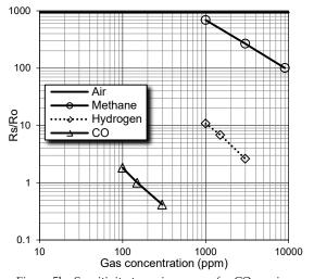
Figure 5b - Sensitivity to various gases for CO sensing (Ro = Rs in 150ppm of CO,  $V_{\rm H}$  =0.2)
