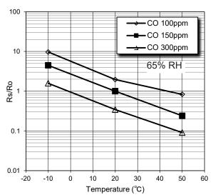
Figure 6b - Temperature dependency for CO sensing (Ro = Rs in 150ppm of CO at  $20^{\circ}$ C/65%RH, VH =0.2)
