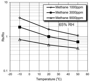
Figure 6a - Temperature dependency for methane sensing (Ro = Rs in 3000ppm of CH4 at 20°C/65%RH, VH =0.9)
