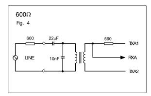
Insertion Loss: 1.8dB @ 2kHz
