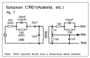
Insertion Loss (Line to RXA): 2.2dB @ 2kHz Frequency Response : ±0.5dB 50Hz – 4kHz
