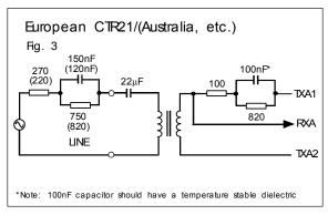
Insertion Loss: 1.0dB @ 2kHz
