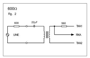
Insertion Loss: 1.8dB @ 2kHz
