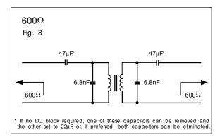
Insertion Loss: 1.5dB @ 2kHz
