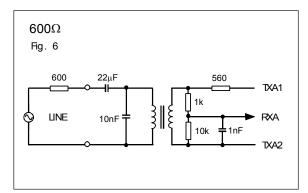
Insertion Loss (Line to RXA): 2.8dB @ 2kHz Frequency Response : ±0.2dB 30Hz – 10kHz
