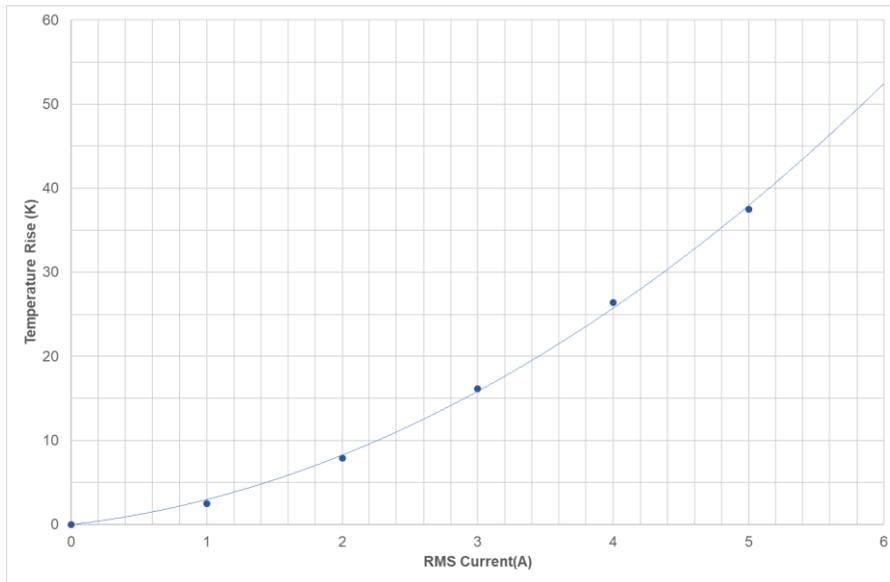
**Fig 12: Temperature rise in DMF4B5R5G105M3DTA0 with RMS current**
