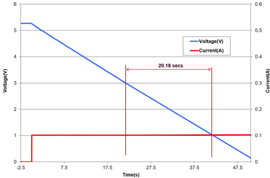
**Fig 2: Measurement of DC Capacitance for a DMF4B5R5G105M3DTA0**
