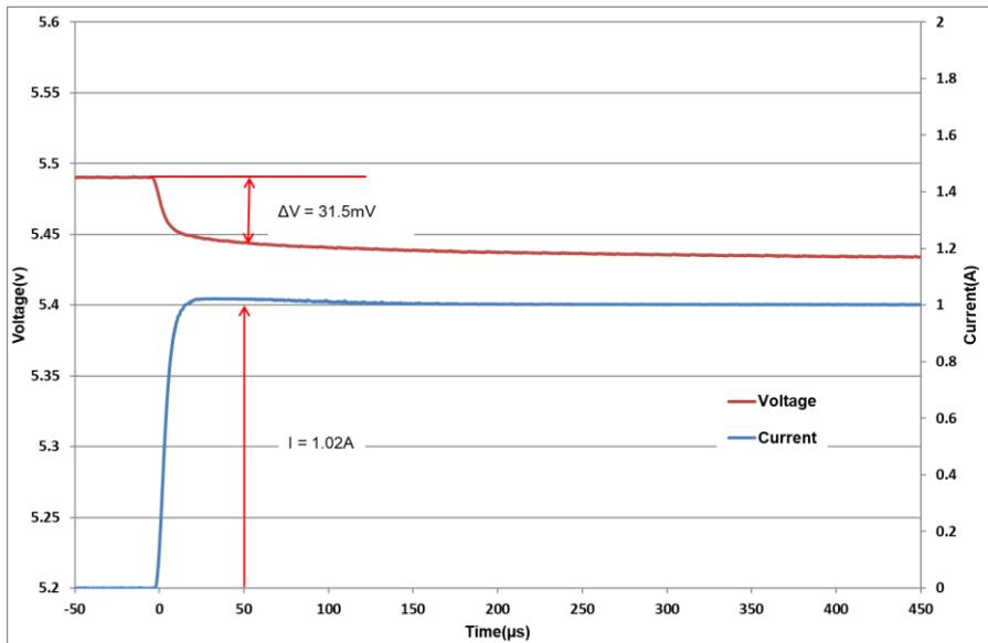
**Fig 3: Measurement of ESR for a DMF4B5R5G105M3DTA0**
