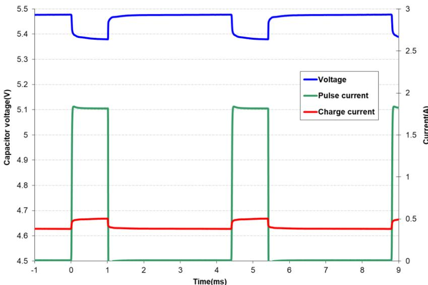
Fig 5 shows that the DMF supercapacitor does an excellent job supporting a GPRS class 10 pulse train, drawing 1.8A for 1.1ms at 25% duty cycle. The source is current limited to 0.6A and the supercapacitor provides the 1.2A difference to achieve the peak current. At first glance the freq response of Fig 8 indicates the supercapacitor would not support a 1ms pulse, but the  $C_{eff}$  of 60mF coupled with the low ESR supports this pulse train with only ~90mV droop in the supply rail.
