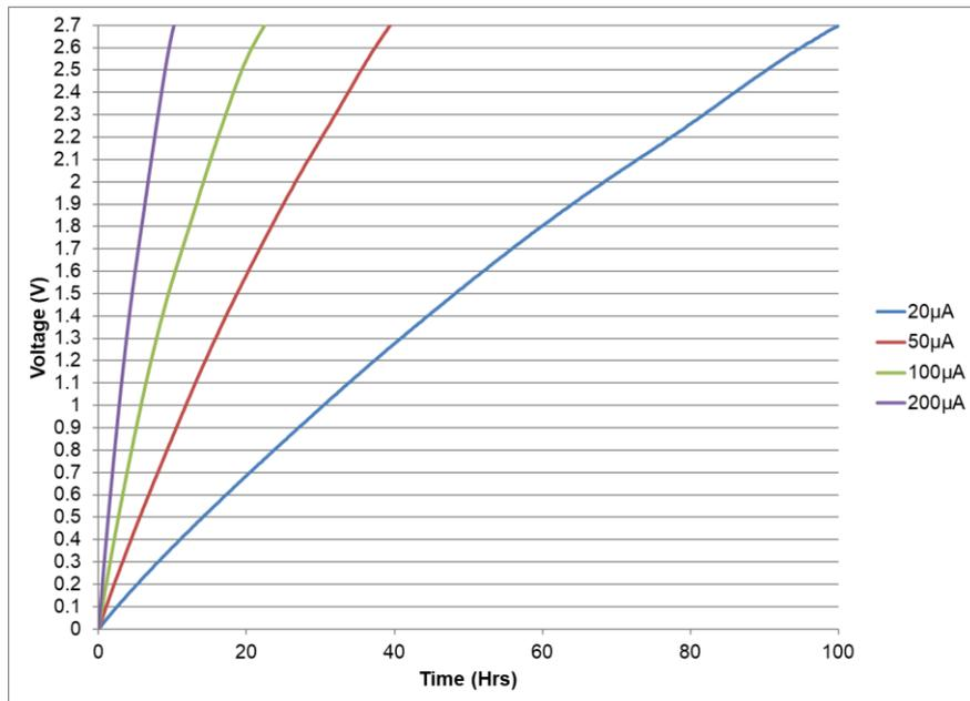
**Fig 11: Charging a single cell of DMF4B5R5G105M3DTA0 (single cell: 2F) with low current**
