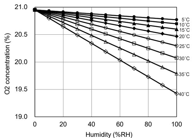
Fig. 6 - Effect of humidity on O2 concentration
