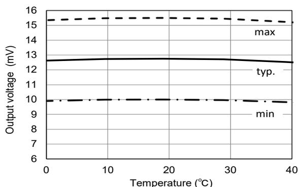
Fig. 7a - KE-25LF temperature dependency of output voltage
