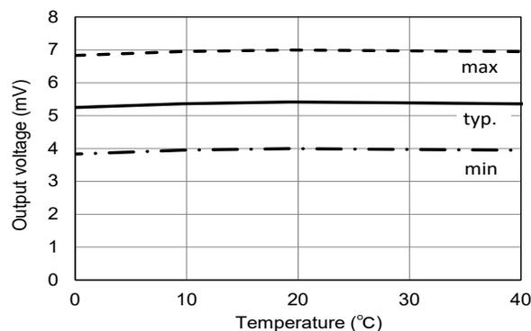
Fig. 7b - KE-50LF temperature dependency of output voltage
