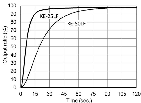
Fig. 4 - Response speed of KE-LF sensors to oxygen
