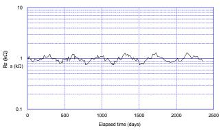
Fig. 14 - Influence of unenergizing on TGS2610-C
