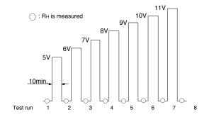
Fig. 21 - Test procedure for heater durability
