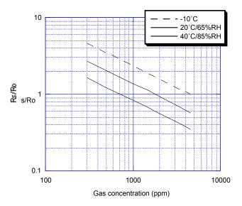
Fig. 7 - Sensor resistance under various ambient conditions
