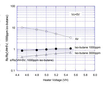
Fig. 8 - Heater voltage dependency (Vc=5.0)
