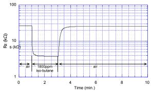
Fig. 10 - Gas response to iso-butane of TGS2610-C
