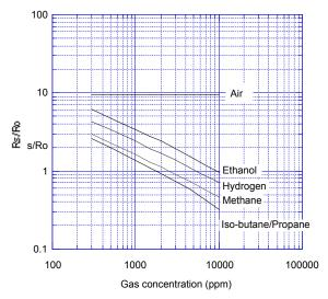
Fig. 4a - TGS2610-C00 sensitivity to various gases (Rs/Ro)
