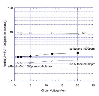
Fig. 9 - Circuit voltage dependency (VH=5.0)
