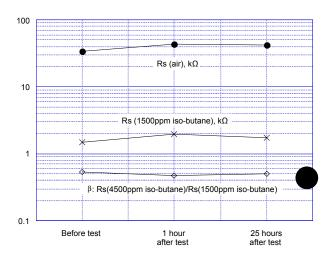
Fig. 18 - Effect of 10% ethanol exposure on TGS2610-C
