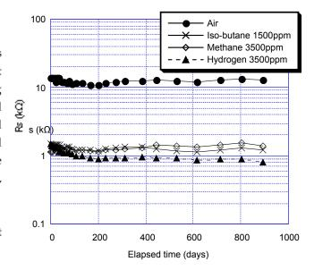
Fig. 13 - Long-term stability (continuous energizing) of TGS2-  $\,$  610-C
