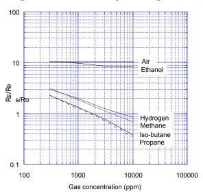
Fig. 4b - TGS2610-D00 sensitivity to various gases (Rs/Ro)
