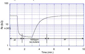
Fig. 10b - Gas response to iso-butane of TGS2610-D
