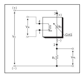
Fig. 2 - Basic measuring circuit
